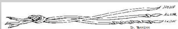
Universal mordant knots help identify results post dye-pot. Drawing by Dorothy Beebe
